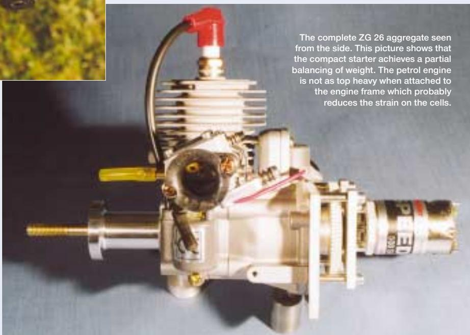
The complete ZG 26 aggregate seen from the side. This picture shows that the compact starter achieves a partial balancing of weight. The petrol engine is not as top heavy when attached to the engine frame which probably reduces the strain on the cells.
