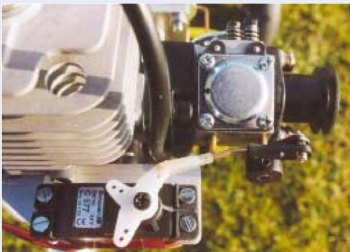
Absolutely recommendable is the choke flap control via the radio transmitter. Although the servo is just beside the ignition cable the DS 20 PCM receiver is not disturbed. A better solution is the control from the fuselage. This is easily possible when using an aspiration manifold by Toni Clark.
